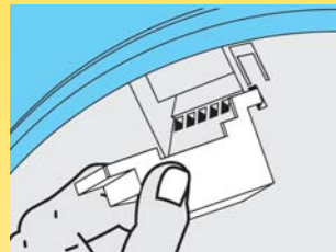
Remove safety cover, wire into alarm
